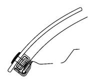
14. Peel and fold two (2) of the large anti-abrasion film pads in half over the hood edge aligned with the inner holes of the deflector in the area above the headlights.
