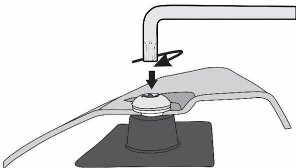
16. Ensure the hood protector is centered on the hood and using a T45 Torx key, tighten the screws into the pedestals. Start in the centermost positions and work outwards. Ensure the shoulder washers are seated properly. Do not overtighten.
