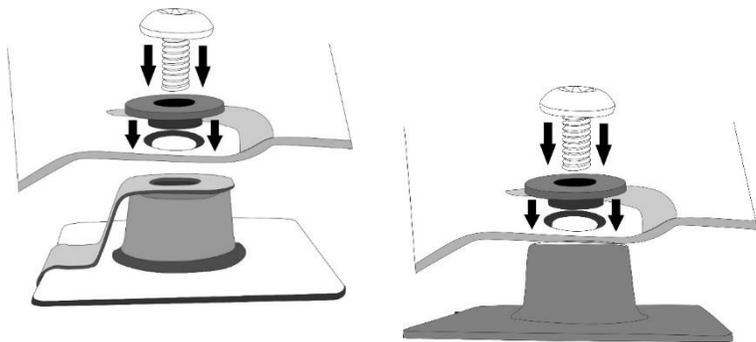
15. Place a Torx head screw through a shoulder washer and into each hole in hood protector. Ensure the shoulder portion of the washer slides into the hole in the hood protector. Loosely thread the screw into the mounting pedestal. See illustration for orientation of the shoulder washer. Repeat for all locations.
