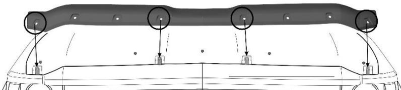
1. Use one of the surface wipes provided and wipe down the area (approximately 15cm (6 in.) from the hood edge) where the hood protector will be installed. Wipe dry with a soft cloth or paper towel. This will remove any wax or grease and will ensure a cleaner surface for the adhesive to bond to.
