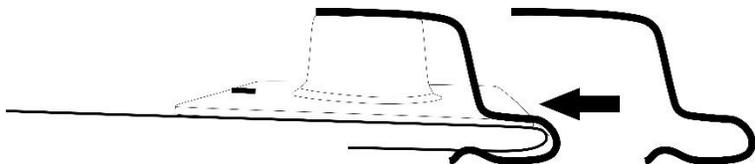
14. Slide metal brackets over the two pedestal positions on each side of the hood and place the hood protector on the bumpers and pedestals.
