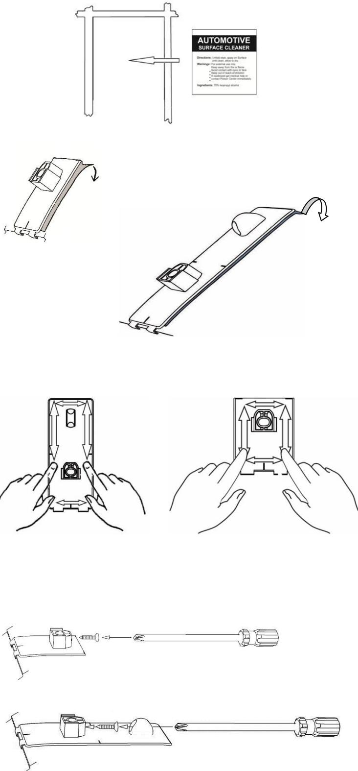
10. Remove the pedestals and thoroughly clean the outlined area with the alcohol wiping pad. Wipe dry with a clean cloth or paper towel. This will insure all wax, finger prints and oils are removed from the hood surface in the bonding area.
