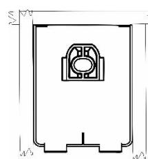
5. Using the repositionable tape strips, temporarily attach the two (2) small adhesive pedestals at the location indicated in the illustration.
