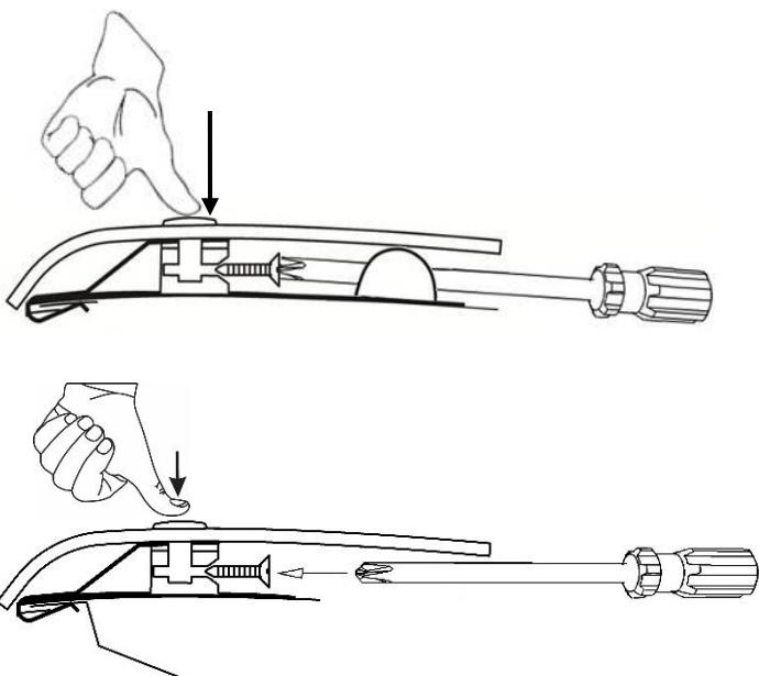
16. Starting at the center location tighten all the screws that were loosely installed in step 15. To ensure proper seating of the components, maintain slight pressure on the pin while simultaneously tightening the screw. Repeat for all remaining pedestal locations.
