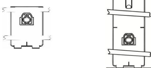
1. Mount four (4) bumpers as indicated in the illustration. **Note:** bumpons must be mounted to the hood surface. If they are mounted to the hood protector they will wear through the paint.
