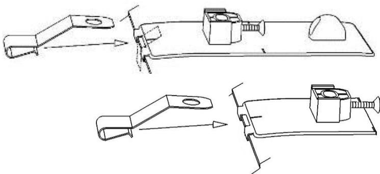
14. Push metal mounting brackets over the hood edge aligned with the anti-abrasion pads installed previously. Ensure each bracket is fully engaged over the hood edge and the hole in the bracket is aligned with the hole in the pedestal.
