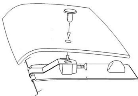
**NOTE:** Only tighten screws a few turns so the pins are held in place but there is still some movement of the protector as this assists in final alignment of all attachment positions.
