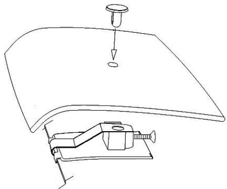
15. Place the protector on the pedestals and, starting at the center location, install a pin through the protector and into the pedestal. Maintain slight pressure on the pin to ensure proper seating of the components, while simultaneously tightening the screw a few turns. Repeat for remaining pedestal locations.
