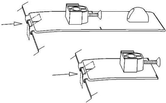
13. Peel and fold an anti-abrasion pad in half over the hood edge between the fingers on each pedestal.
