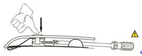
17. Maintain slight pressure on the pin, to ensure proper seating of the components, while simultaneously tightening the screw.
