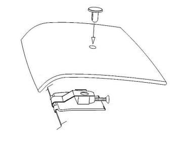
18. At the four (4) small pedestals, drop a pin through the protector and into the pedestal.
