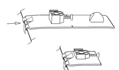
13. Peel and fold the small anti abrasion film pad in half over the hood edge between the fingers on the pedestal.
