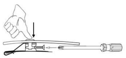
19. Maintain slight pressure on the pin, to ensure proper seating of the components, while simultaneously tightening the screw.
