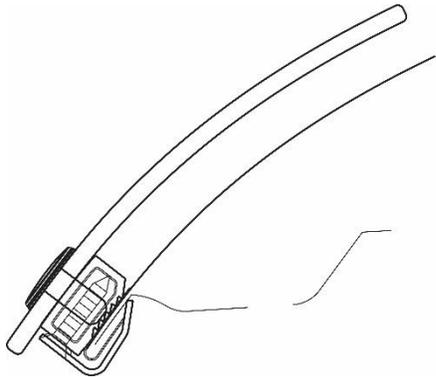
19. Ensure the hood protector is centered on the hood and using a T45 Torx key, tighten the screws into the pedestals. Start in the center position and work outwards. Ensure the shoulder washers are seated properly. Do not overtighten.
