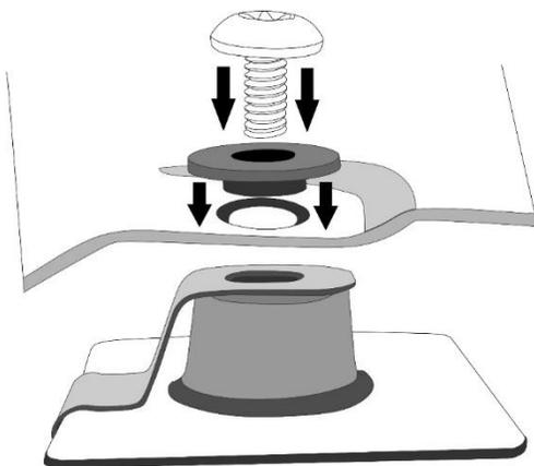
15. Peel the red protective backing off one of the adhesive pedestals. Carefully place it on the hood surface exactly where the tape outline is. **Use care with this step as once the pedestal has been placed on the hood, it will be very difficult to remove.** Repeat for all locations.
