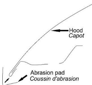
1. Use one of the surface wipes provided and wipe down the area (approximately 15cm (6 in.) from the hood edge) where the hood protector will be installed. Wipe dry with a soft cloth or paper towel. This will remove any wax or grease and will ensure a cleaner surface for the adhesive to bond to.
