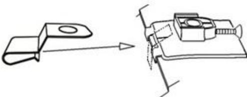
13. Place the protector on the metal brackets. Align the 4 center most holes in the protector with the holes in the metal brackets. Install a "push type retainer" through the hole in the protector, and into the bracket. Ensure the protector is seated against the metal bracket and push the center pin of the retainer assembly to lock it into place. Repeat for 3 remaining positions.
