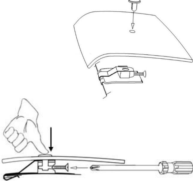
14. At the 2 outermost locations, install a pin through the protector and into the pedestal.
