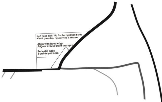
2. Cut out and tape the "Pedestal locating template" (found on page 6) to the left hand edge of the of the hood as shown.
