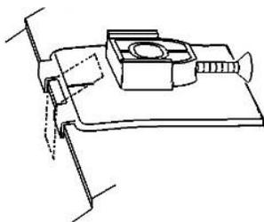
12. Push a type C metal mounting bracket over the hood edge. Align the hole in the bracket with the hole in the pedestal.
