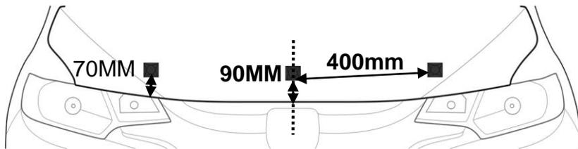
1. Install the three (3) Bumpons as shown. **Attention: the Bumpons must be installed on the hood, not on the protector!!!** If the Bumpons are installed on the protector, they may wear through the paint.
