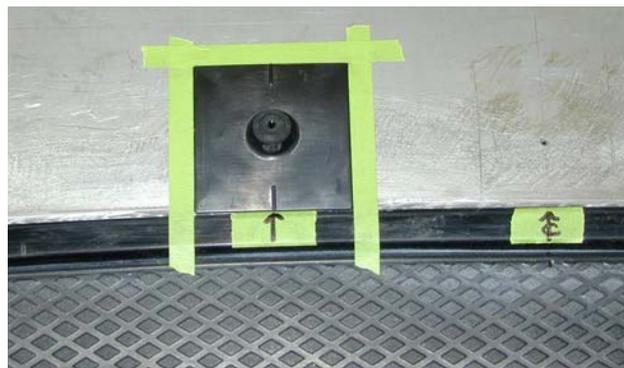
5. Temporarily tape the pedestals to surface of the hood in their determined positions, confirm correct placement by placing the hood protector on top of the four pedestals. When positioned correctly the four (4) holes in the center area of the protector will align with the holes in the expansion plugs. Adjust if necessary and reconfirm the pedestal locations using the measurements in the illustration and the hood protector.
