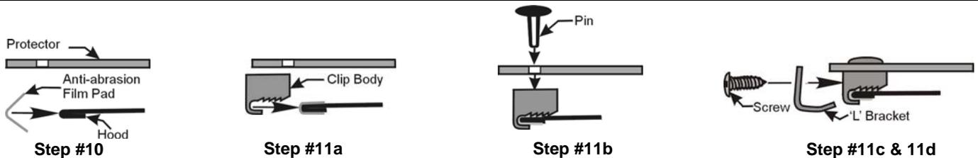
12. On some vehicles it may be necessary to adjust the hood bumpers and/or latch for proper clearance. **Note: Do not pull on the protector when opening or closing the hood.**
