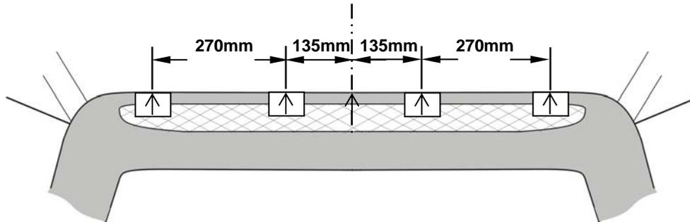
4. Install the square expansion plugs into the top of the adhesive backed pedestals. Use the centering notch on the pedestals to align it's location with the pencil mark on the tape in the previous Step. **Note:** When located correctly the pedestal leading edge will butt against the back of the grill surround at all 4 locations. See *Illustration*.
