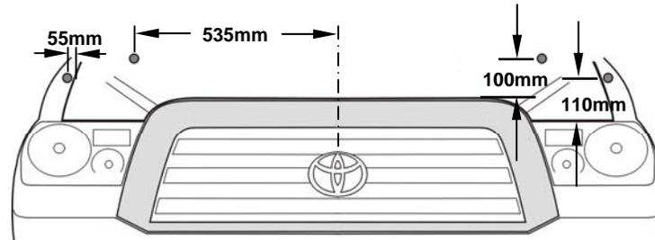
9. Place the hood protector on the hood and fasten the (4) # 8 x 7/16" truss head screws through the protector and into the expansion plugs. **Do not over-tighten.**
