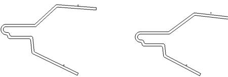
4. Install the Metal Brackets over the hood edge in their correct location, aligning the hole in the bottom leg of the bracket with the round hole in the hood.
