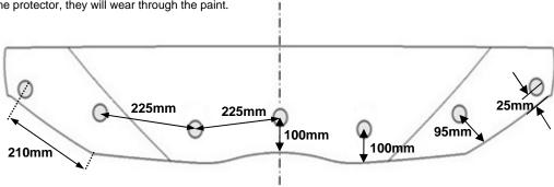
3. Open the hood of the vehicle. Peel and fold anti-abrasion film pads in half over the edge of the hood, in the four (4) locations shown. Center the film pads with holes identified in the illustration.
